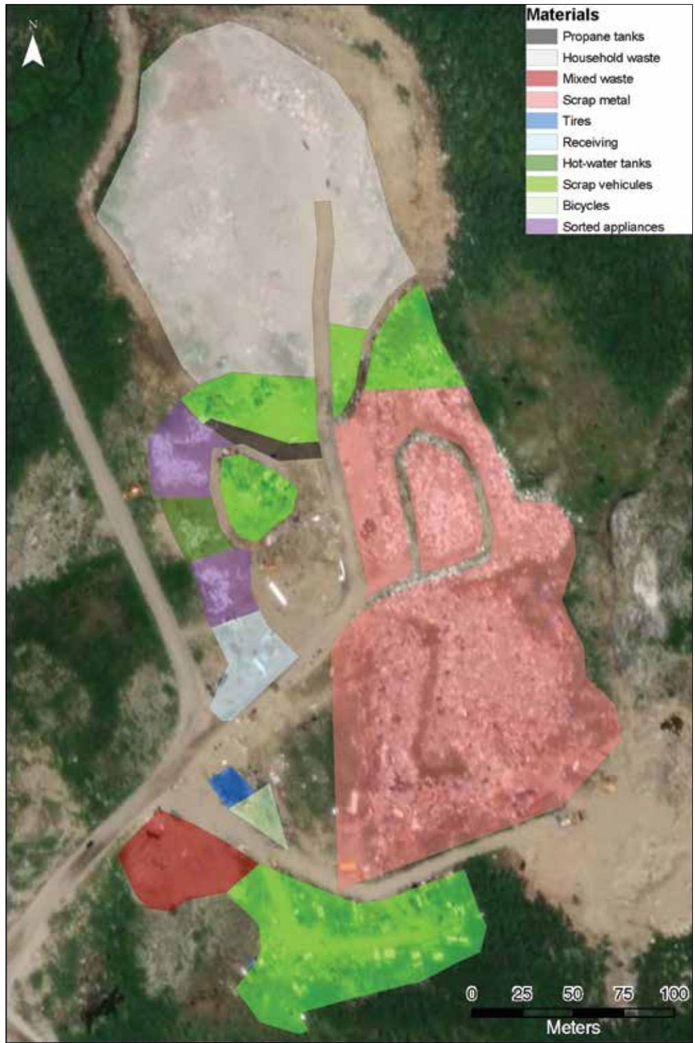
Figure 15: Storage zones for non-combustible residual materials at the northern landfill in Kuujuaq
