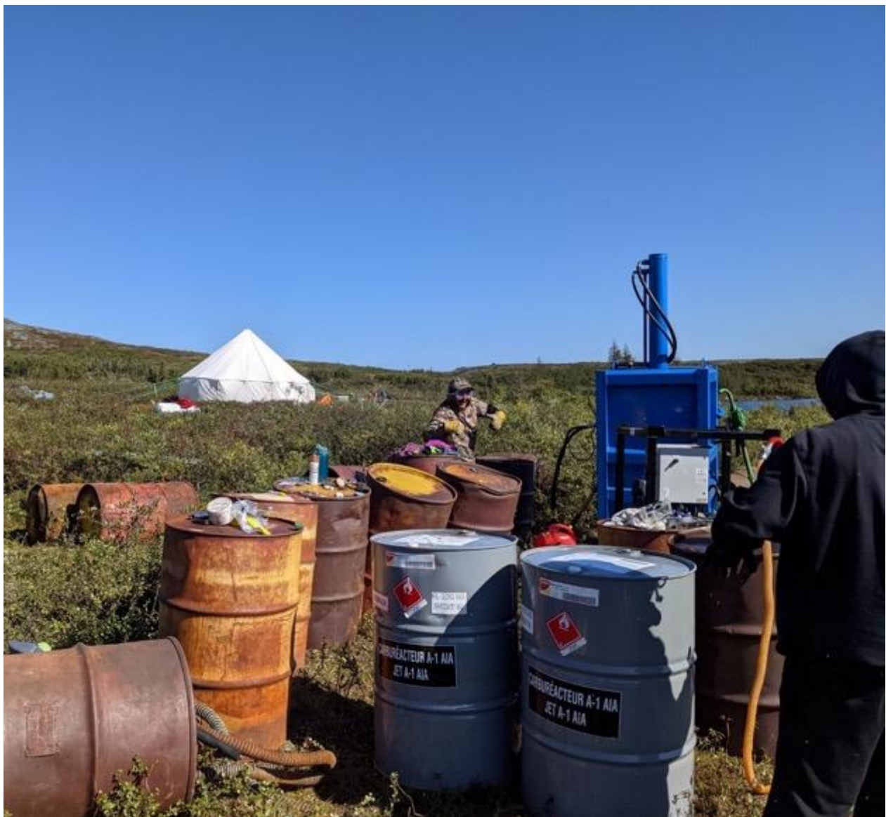
Figure 24 Pumping and crushing drums at Gerido-5
