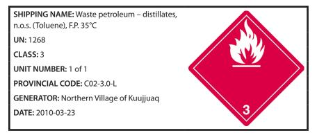
**Used antifreeze** should be stored in closed plastic or metal drums. For transportation purposes, up to four drums may be secured to a pallet. Labels (see immediately below) should appear on all drums.
