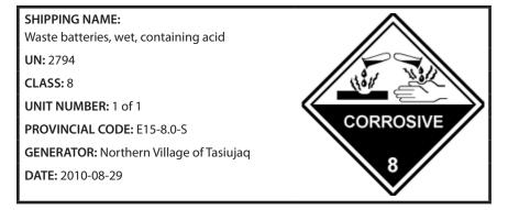
**Batteries** may be stored in open plastic drums. Metal drums may also be used with an inserted plastic liner since batteries contain corrosive acids. The general public should be encouraged to dispose of their batteries in these drums at a designated location rather than as regular trash at the local residual materials disposal site. Labels (see immediately below) should appear on all drums. A UN-certified container may also be required.
