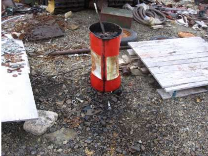
Figure 57: Site K-61. Barrel containing grease along with other debris (circled in yellow in Figures 49 and 50). Petroleum-hydrocarbon soil contamination.
