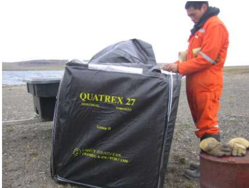
Figure 150: Site SW-34. Batteries to be carried by helicopter sling in a specially designed bag.
