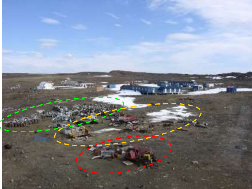
Figure 49: Site K-61 in 2007. The renovated Expo Camp is shown in the background (old and new buildings). Debris observed at site K-61 during the 2001–2002 inventory is shown circled in yellow. Debris gathered from minor and intermediate sites is shown circled in red. Recent barrels deposited by Canadian Royalties are shown circled in green.
